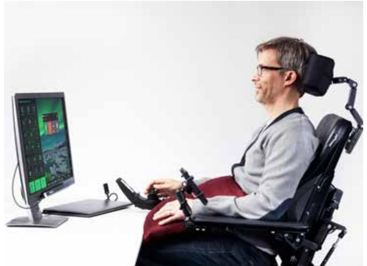
we have further improved the look and feel of the hardware to align the PCEye Plus with the silver/black color theme of the Tobii Dynavox family. The back of the eye tracker is made from magnesium, which is optimal for heat distribution and reduces the weight. The two-part design of the front gives the device a very modern look and emphasizes the microphone slot, which stands out visually from other eye trackers.
